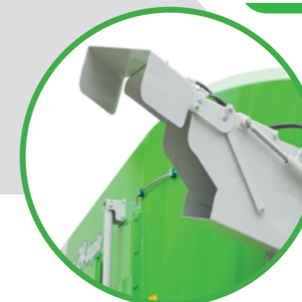
Detalle visera orientable 30 + 30°
